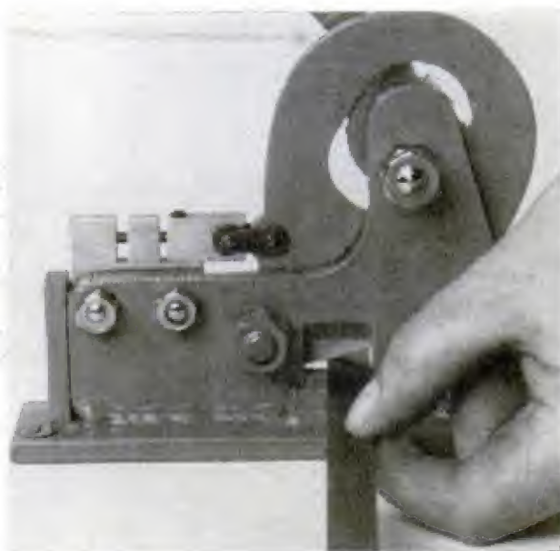
PUNCH ALSO ACTS AS SHEAR for cutting the metal strips. Sharpened lower edge works like a guillotine
